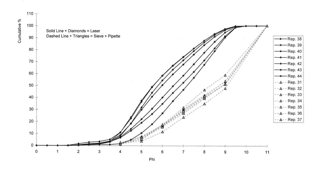
Figure 2. Particle size distribution curves resulting from analysis of replicate samples of sediment distributed as PS11. Seven samples analysed by sieve-pipette and seven samples analysed by Laser.
