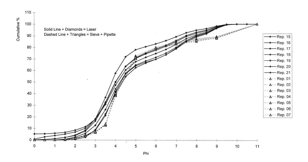
Figure 3. Particle size distribution curves from participating laboratories for sediment samples from PS10. The average values for the AQC analysis of replicates are included.
