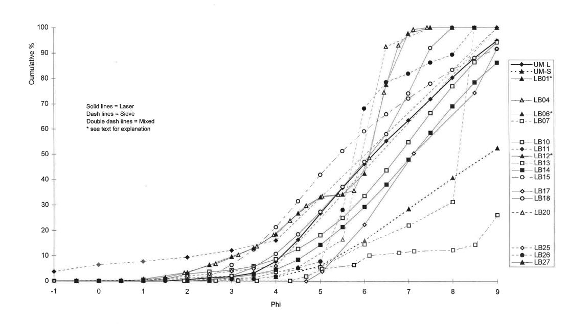
Figure 4. Particle size distribution curves from participating laboratories for sediment samples from PS11. The average values for the AQC analysis of replicates are included.
